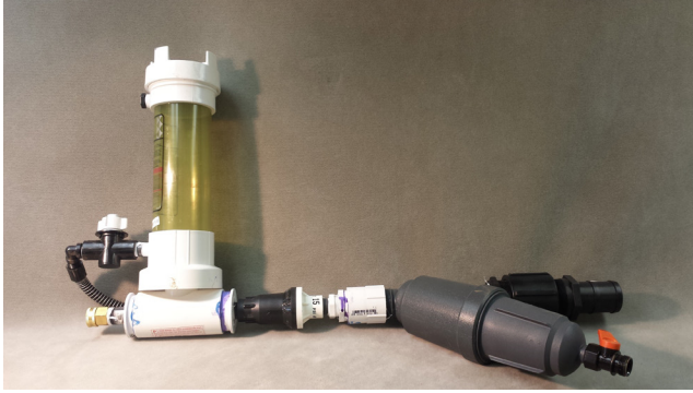
Figure 7. Injector system to add fertilizer through irrigation lines. (Photo by Stephen Stanphill)
